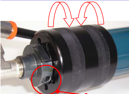
USE THIS SCREW TO ADJUST THE TENSION FORCE VALUE
