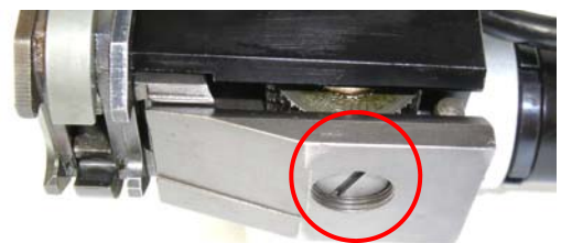
TURN THIS TO ADJUST THE GAP BETWEEN THE FEEDWHEEL AND THE PRESSURE BUTTON
