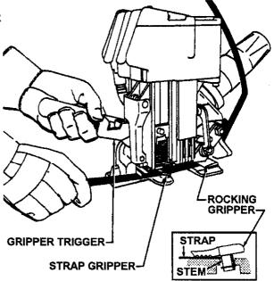
2. Insert the top strap between the feedwheel and the rocking gripper and insert it into the slot of the strap latch. Pull excess slack from the strap. Make sure you are not standing in line with the strap and press the tensioner lever all the way down. It will lock in place. The feedwheel will engage automatically and the tool will begin tensioning. Should it become necessary to stop the tensioning cycle, press the valve latch forward.
