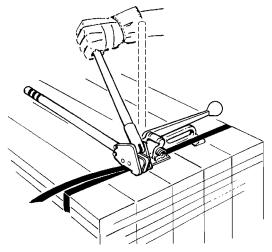
2. Bring sealer handles completely together to assure a proper notch.
