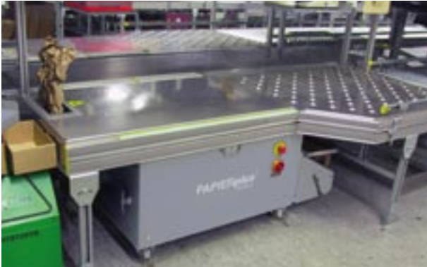
Example of a PAPERplus® Classic tabletop machine integrated in a packaging line.
